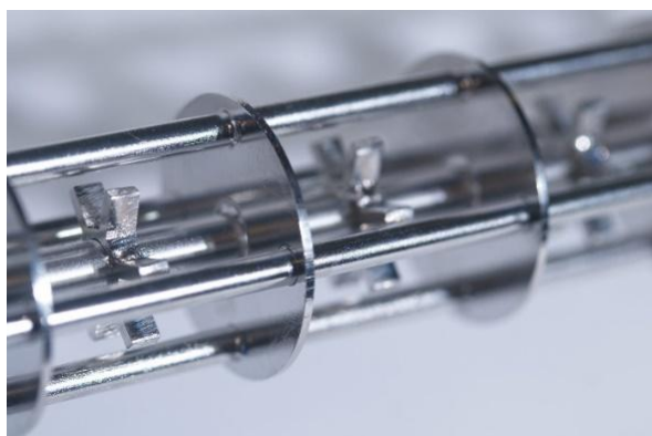
Figure 2 – Detailed image of each individual CSTR with its internal agitator
