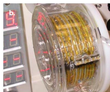
Figure 6. Using the 'Dual-Core™' tubing reactor for reaction optimization. (a) 810 µL reactor. (b) 10.2 mL reactor.
