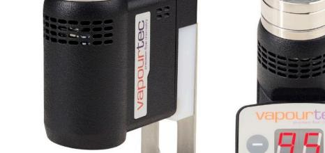
The Vapourtec eBPR is an electronically adjustable back pressure regulator designed for precision and versatility in flow chemistry applications. It controls pressures from 0.5 to 20 bar, without the need for an external reference gas pressure. Made with only PTFE and PFA wetted parts to ensure chemical compatibility, it allows precise pressure control over a range of working fluid temperatures up 100 **Learn More**
