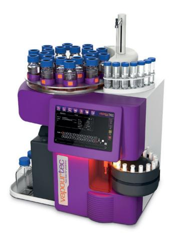
In 2017 Vapourtec developed the Variable Bed Flow Reactor (VBFR). the key technology enabling Fast-Flow peptide synthesis. the VFBR maintains the swollen resin at a constant packing density, minimising its volume, thereby eliminating channelling of reagents and solvents and maximising washing efficiency.
