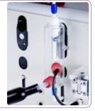
Gas/Liquid "tube-in-tube" reactor
