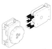
The **Stand-alone** version of the Ion is designed for use in conjunction with your Vapourtec system or with 3<sup>rd</sup> party pumps and power supply. This version does not include the parts that allow temperature control of the reactor. In other respects, the stand-alone version is identical to the integrated version using identical electrodes and membranes.
