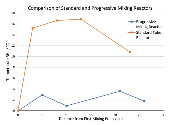
It is clear that when using a reactor with a single mixing point a temperature rise of almost 17 °C occurs, whereas under the same conditions the Progressive Mixer reactor reduces the rise to less than 4 °C. We believe this enhanced control will enable the chemist to access these high-energy reactions with the confidence that the Vapourtec Progressive Mixing Reactor will prevent localised high temperatures.
