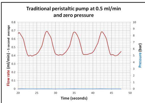
A standard peristaltic pump gives quite significant flow rate fluctuations. This is especially important with two pumped reagents – if these flow fluctuations were out of phase there would be huge swings in reaction stoichiometry entering the reactor.
