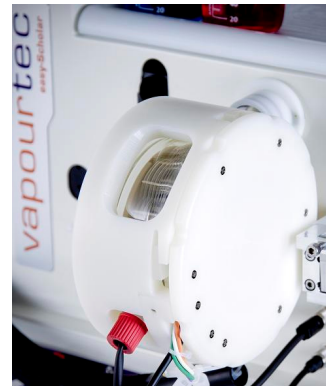
Cooled reactor (-70°C)
