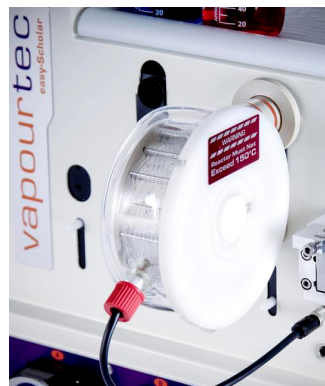
Standard reactor (+150°C)
