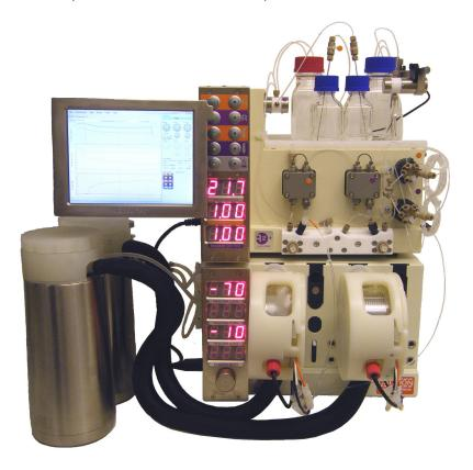
R Series shown with two cooled reactors, running at two different temperatures.
