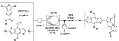
A selection of conjugated polymers, widely studied in organic electronics, was synthesised using continuous flow methodology. As a result of superior heat transfer and reagent control, excellent polymer molecular mass distributions were achieved in significantly reduced reaction times compared to conventional batch reactions.
