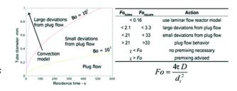
Continuous flow chemistry is being used increasingly; however, without detailed knowledge of reaction engineering, it can be difficult to judge whether dispersion and mixing are important factors on reaction outcome. Understanding these effects can result in improved choices of reactor dimensions and give insight for
