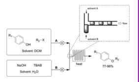
O-Alkylation of phenol compounds was performed in a continuous flow apparatus
