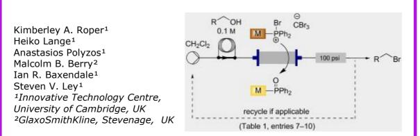
Herein we describe the application of a monolithic triphenylphosphine reagent to the Appel reaction in flow-chemistry processing, to generate various brominated products with high purity and in excellent yields, and with no requirement for further off-line purification.
