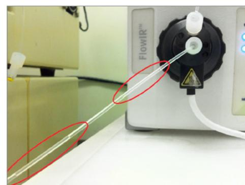
**Figure 9.** Carbon dioxide bubbles (marked) seen entering FlowIR™. No effect on the detected signal was observed under these challenging conditions.
