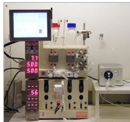
**Figure 2.** The reactor setup consisting of the Vapourtec R2 pump module and R4 reactor module along with METTLER TOLEDO FlowIR™
