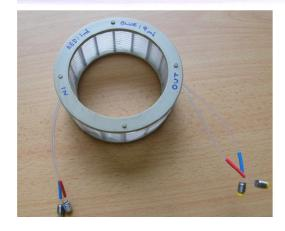
The Dual Core<sup>™</sup> cartridge is a simple drop in replacement for the standard cooled reactor coil usually supplied with the cooled reactor
