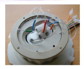
Plumbing the colour coded tubes into the cooled reactor manifold is straightforward
