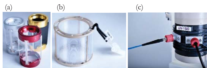
Figures 4. (a) Selection of glass-filter inserts, (b) 10 mL-FEP reactor coil and (c) fiber-optic probe and temperature sensor attachments.
