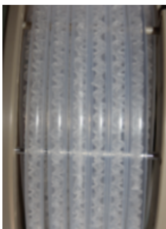
Large diameter reactor with full-length mixing elements
