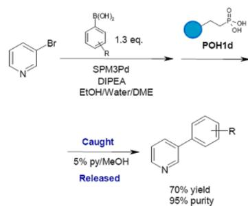
**Figure 11. 'Catch and release' SPE purification of 3-phenylpyridine using POH1d**
