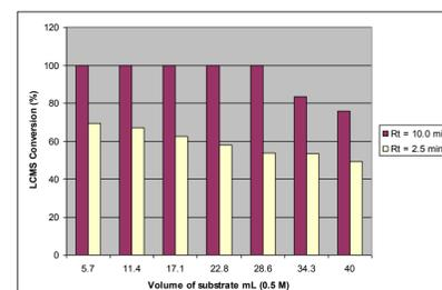
**Figure 8. Study of conversion dependence on continuous Suzuki Reaction of 3-bromopyridine with phenylboronic acid at 130 °C with R<sub>t</sub> 10.0 mins and R<sub>t</sub> 2.5 mins**
