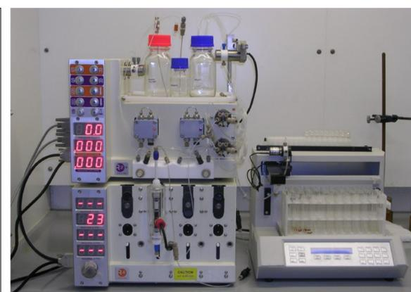
**Fig 4 Vapourtec R Series System with fraction collector**
