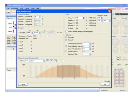
**Fig 5 Setup and control of reaction parameters using Vapourtec Flow Commander™ software**
