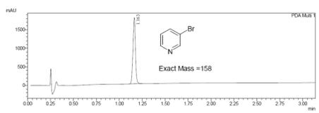
**Figure 10. a) HPLC chromatogram (UV<sub>215</sub> nm) of the 3-bromopyridine starting material**
