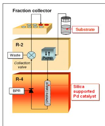
**Fig 3 Flow System Setup**
