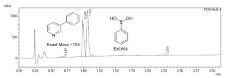
**Figure 10. b) HPLC chromatogram (UV<sub>215</sub> nm) of 3-phenylpyridine crude reaction product**
