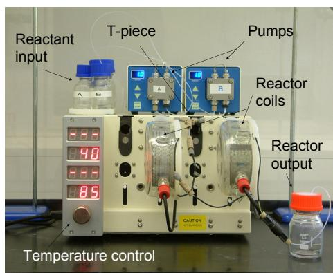
During a 10 week trial, chemistry was conducted on the Vapourtec R4 to assess its usability and utility in a medicinal chemistry environment.
