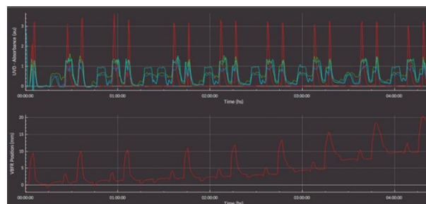
Figure 8 - VBFR volume change (orange) and UV (blue) data over time for the synthesis
